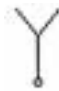
Could be nocking point to high move down slightly if it gets worse try the other direction. If this can not correct the tear pattern and you are a release shooter your arrow spine may be too weak. Go to stiffer arrow or make the bow weight lighter. (If your arrows are long you can cut them shorter to stiffen them.)
